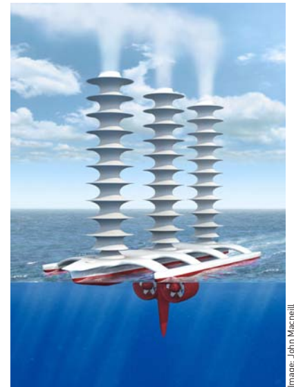
Ships like this concept Flettner vessel could spray sea-water mist into the air to brighten clouds. Thousands of these remote-controlled ships would be deployed to brighten the clouds over large portions of the Earth's oceans.
